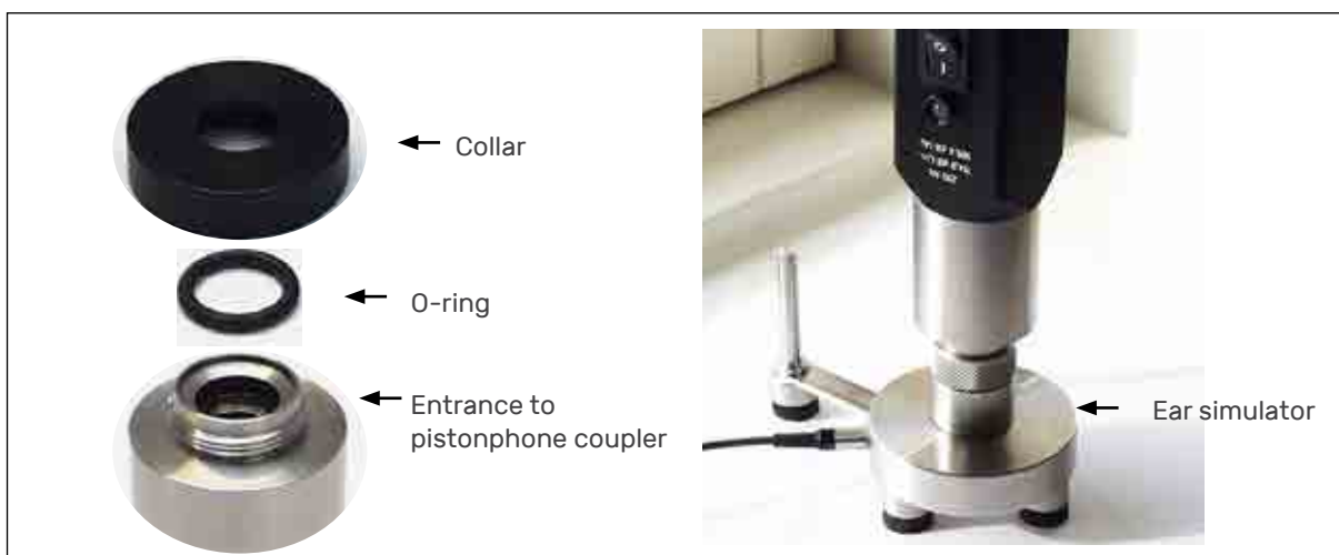
Fig. 4. Calibration using the pistonphone
